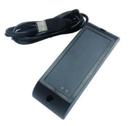
The RFID reader MINI, with protection class IP65, is designed for integration in different applications where robustness is important.
