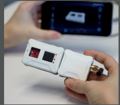
LEGIC XDK Secure Sensor Evaluation Kit with LEGIC Security Module and Secure Element
