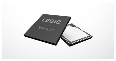
LEGIC inside: the SM-4200 security module supports all relevant RFID standards based on 13.56 MHz such as ISO 14443 A + B, ISO 15693, LEGIC RF, Inside Secure and NFC. Its compact size and patented wake-up circuitry make it the right choice for all kinds of security applications.
